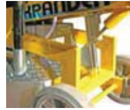
Electric device to adjust the working pressure
